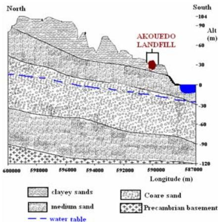
Fig. 2. Geological profile of the Akouedo area
