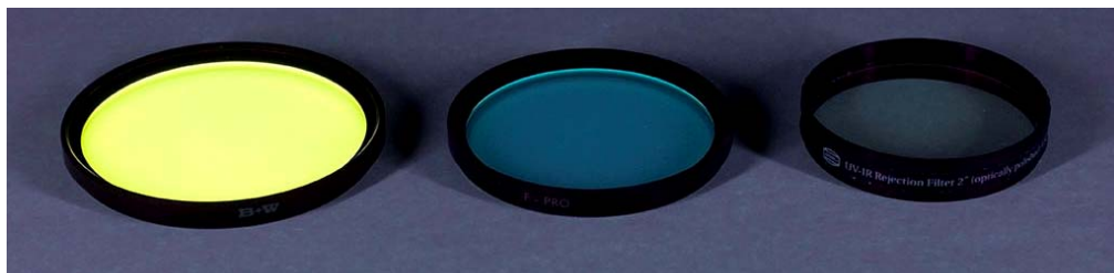
Fig. 1. From left to right: B+W 415 filter, glowing with internal fluorescence; B+W 486 interference filter; Baader UVIR rejection interference filter. Filters receiving direct UV radiation from Wood’s lamps (for other relevant data from image capturing and post-production, please read “Materials and Methods”).
