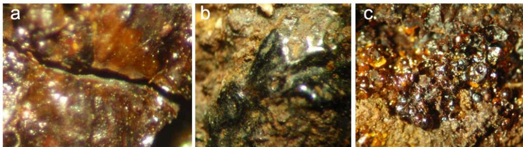
**Fig. 2.** Formations in the corrosion crust (50X): a - coating structures, b - embossed coating formations, c - cracks in the corrosion crust
