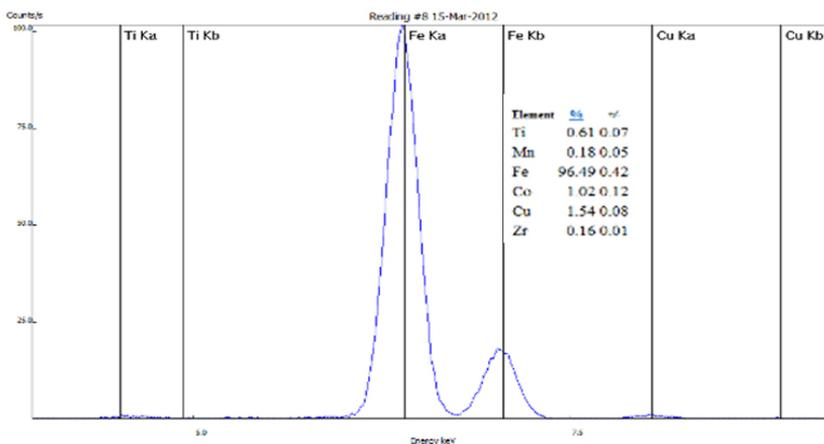
**Fig. 4.** XRF spectrum of the buckle
