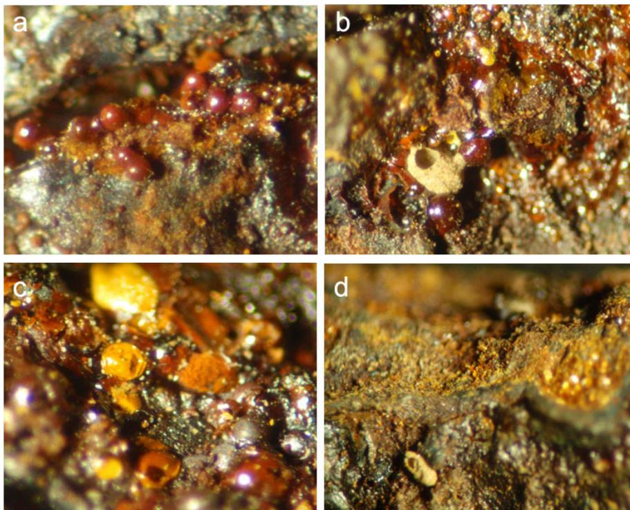
**Fig. 3.** Alveoli formations (50X): a - whole; b - whole and broken; c - broken and monolithized; d - microstructures from the soil
