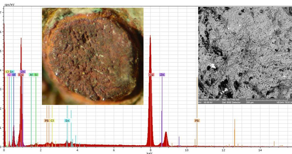
**Fig. 9.** The EDX spectrum, the OM (20X) and SEM image (500X BSE) of the corrosion crust of the nut
