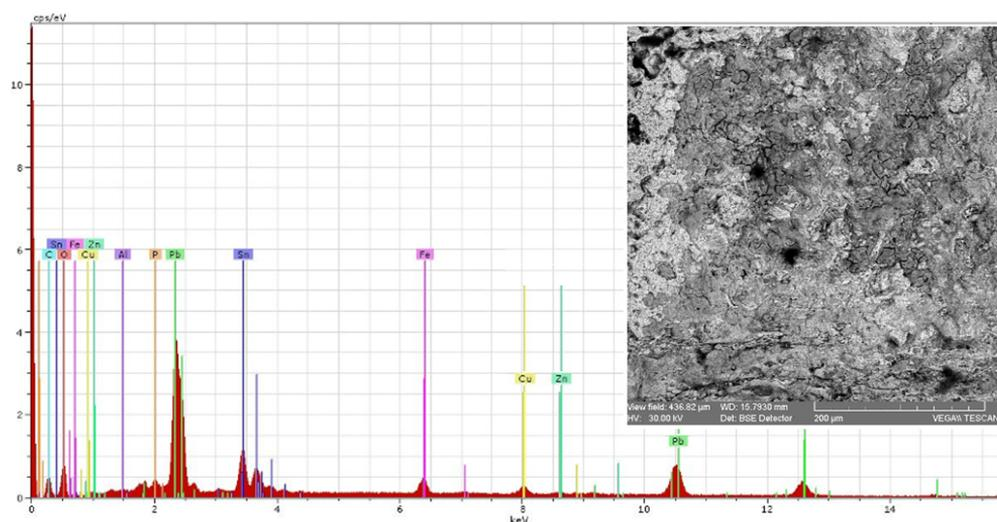
Fig. 6. The EDX spectrum and the SEM image (500X) of the corrosion crust of the pendant
