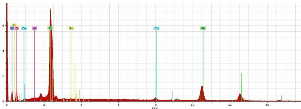
**Fig. 8.** EDX spectrum of the corrosion crust with bead formations
