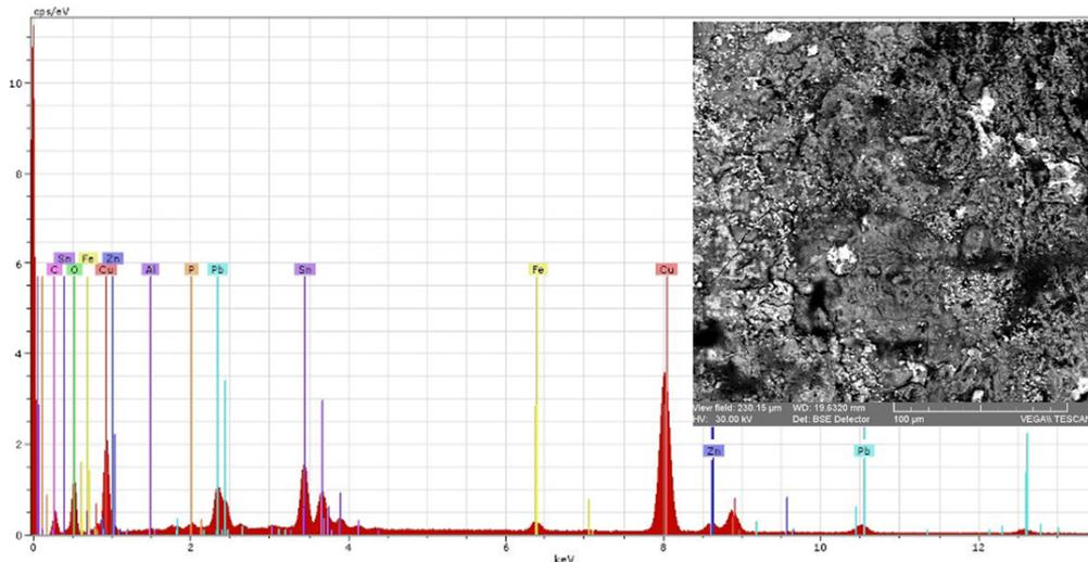
Fig. 10. The corrosion crust near the nut: a - SEM image (500x BSE); b - EDX spectrum
