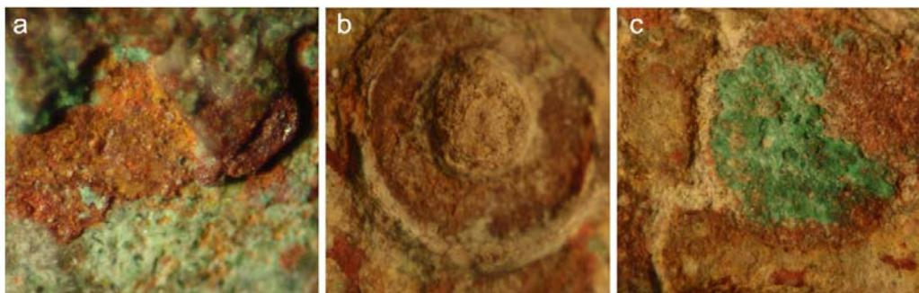
Fig. 5. The morphology of the corrosion crust: a - distribution of the chemical compounds in the corrosion crust, b - microstructures in the corrosion crust, c - pits and craters in the corrosion crust
