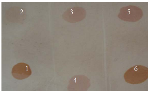
Fig. 5. Removal of red stains produced by S. parvullus using different solvents: 1 - control, 2 - dimethyl formamide, 3 - Ethanol, 4 - doxian, 5 - Diethyl ether, 6 - n -Hexan.
