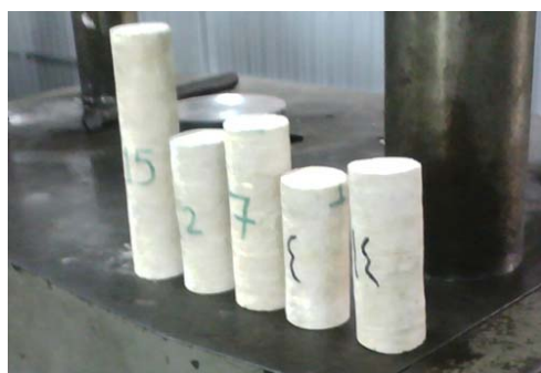
Fig. 5. Some Core Samples after Preparation for Mechanical Testing
