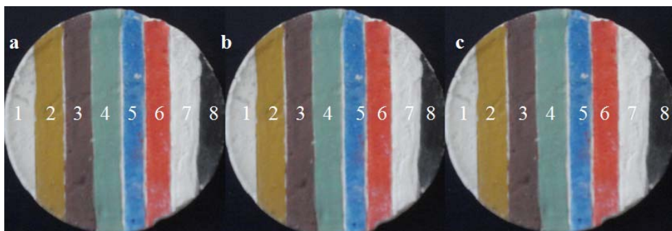
Fig. 7. Color change of pigments after irradiation: (a) Control, (b) 5kGy, (c) 25kGy, (1) gypsum plaster, (2) limonite, (3) hematite, (4) malachite, (5) azurite, (6) vermillion, (7) calcium carbonate, (8) lamp black.
