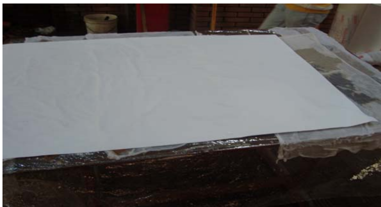
Fig. 15. Drying process by tissue paper
