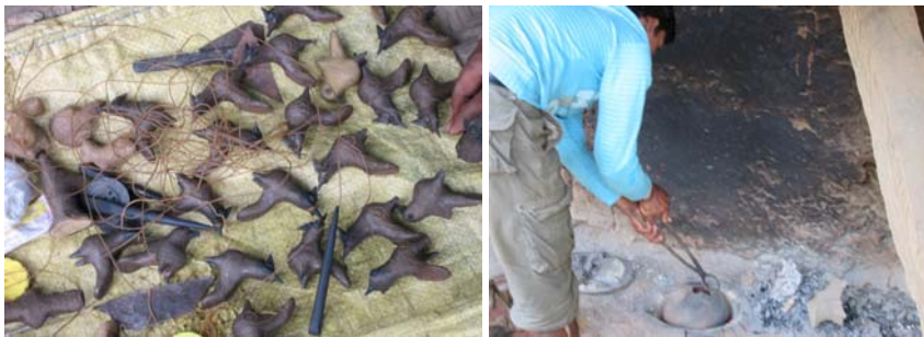
Fig. 3. Wax items under semi-construction and the dhokra metals melted in the fire pit.
