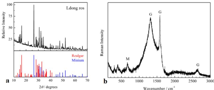
**Fig. 2.** Left: X-ray powder diffraction patterns of the orange pigment Ldong ros showing a mixture of realgar and minium. Right: Raman spectrum of black ink Snag tsha showing a mixture of magnetite (M) and graphite (G).
