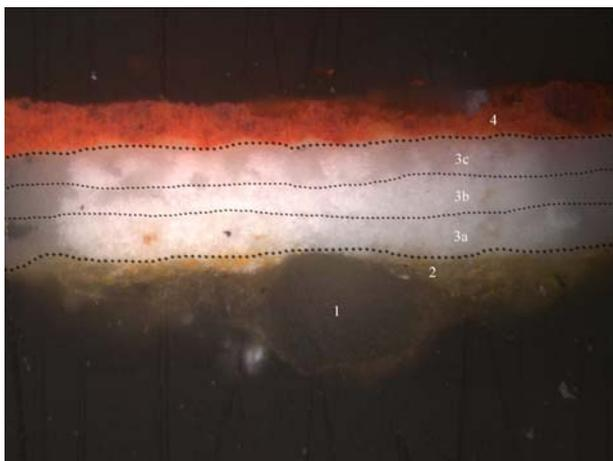
**Fig. 3.** Cross section of spot no 7 shows the layer structure with all the ground layers.
