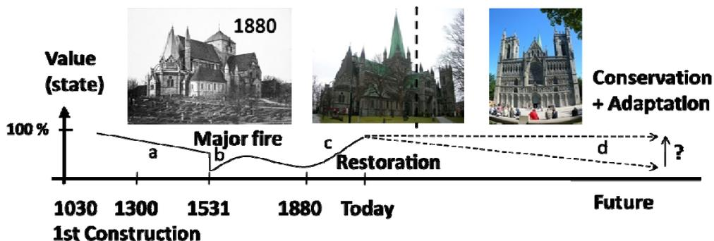
**Fig. 1.** The historical condition of the Nidaros cathedral in Trondheim, Norway, due to lacking maintenance (a), a catastrophic event (b), restoration (c) and future possible scenarios (d). The vertical dotted line distinguishes the front part (photo to the right) which was added during the conservation from the 1880s.
