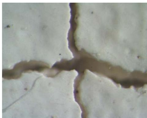
**Fig. 4.** Microscopic photograph of sample C<sub>4</sub> (aged and consolidated with sturgeon glue, on canvas) after the *Thermo Lignum*® Warmair treatment (magnification approx. 55 times)
