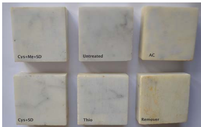
Fig. 6. Stained and cleaned marble specimens
