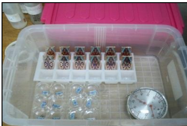
Fig.4. Microclimate used for the test with a hygrometer and temperature measuring device.
