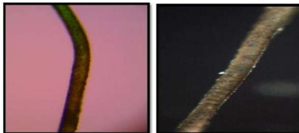
Fig. 6. The microscopic pictures, taken by polarizing microscope, of black yarn taken from the archaeological kilim, which indicate to the missing in scales of wool fibres as a result of ageing inside the museum.
