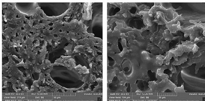
Fig. 4. SEM micrographs of treated (a) *Patanus orientalts-L* samples in PVB solution (A4) and (b) treated in PVB solutions with nano-ZnO additives in 1.0% ZnO, magnification 500X: a and b: cross section: consolidate is visible through vessels and fibers as white bubbles.
