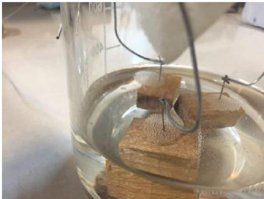
**Fig. 1.** Immersion of wood samples in the consolidate solution
