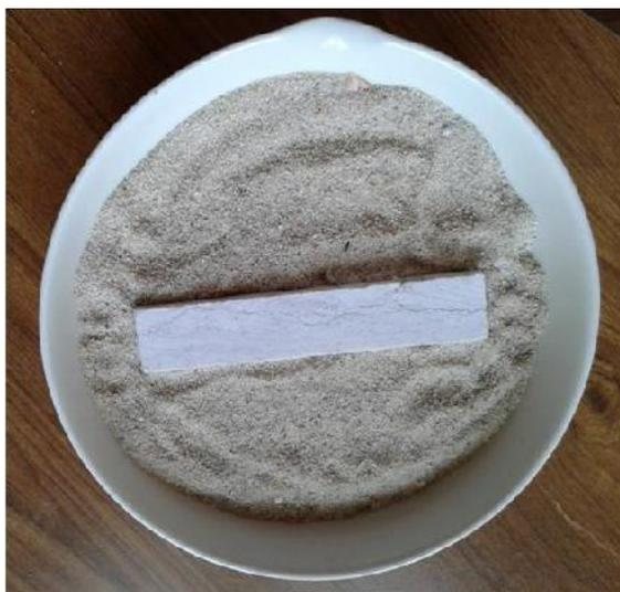
Fig. 2. Sample encased in fine sand.
