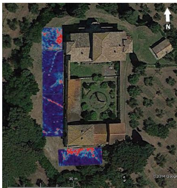
Fig. 6. The relevant red GPR anomalies at about 0.7m depth around Villa Maruffi due to possible buried structures.
