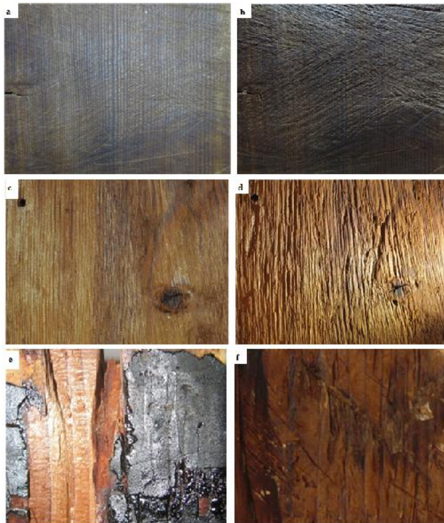
Fig. 6. Images with marks on wood: Saw marks on a sled of shrine GEM-No 21073: a - Flat light; b - Racking light; Marks left by sanding tool inside face of a side board from shrine GEM-No 21062; c - Flat light; d - Racking light; e - Cone shape of dowel hole by bow_drill GEM-No 21046; f - Marks left by adze on the sled of shrine GEM-No 21061
