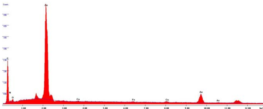
Fig. 8. EDS spectrum of golden leaf present in the cross section of sample A_03
