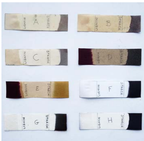
Fig. 1. Spot-tests for acid and alkaline papers. On the left of each sample, lignin detection; on the right, starch detection
