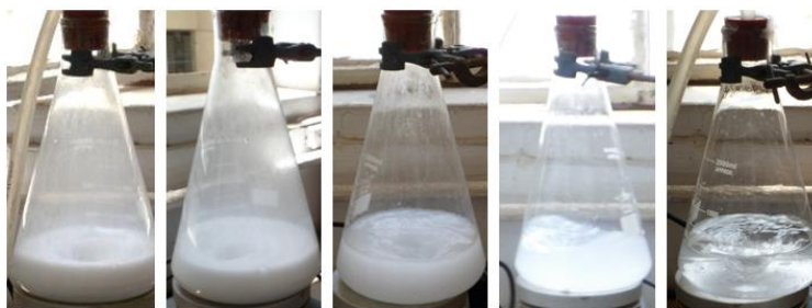
Fig.1. Stages of the preparation of aqueous solution of magnesium Bicarbonate in laboratory
