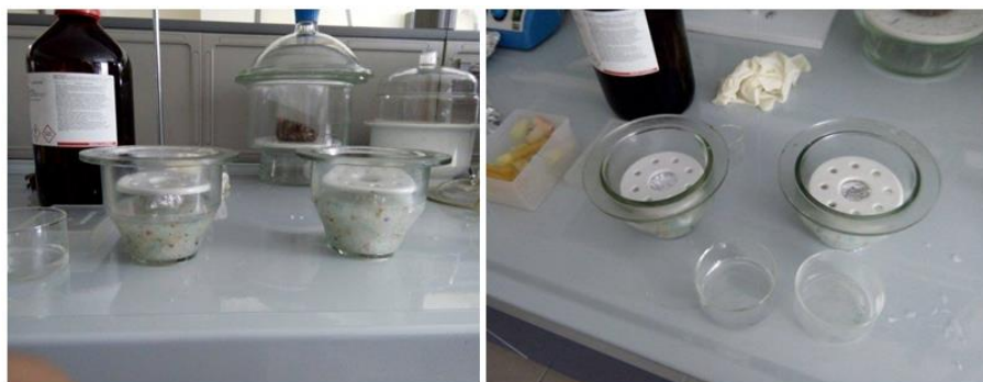
Fig. 4. Two desiccator jars are used for hydrogen peroxide test. Inside each jar small piker was located to contain the filter paper soaked in 5% hydrogen peroxide solution.
