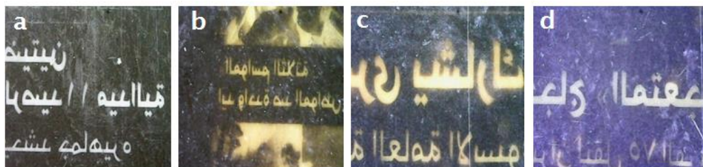
Fig. 6. The oxidized samples: a - Physical decay of the CA controlled samples shows appearing of 'Cinch' marks caused by the action of film moving against itself in the roll; b - CA oxidized sample show the formation of redox blemishes type 4; c - CA sample coated by zinc. It shows the oxidizing of silver particles and forming redox blemishes; d - CA sample coated by copper. It shows a good stability and reducing of oxidizing of silver particles.
