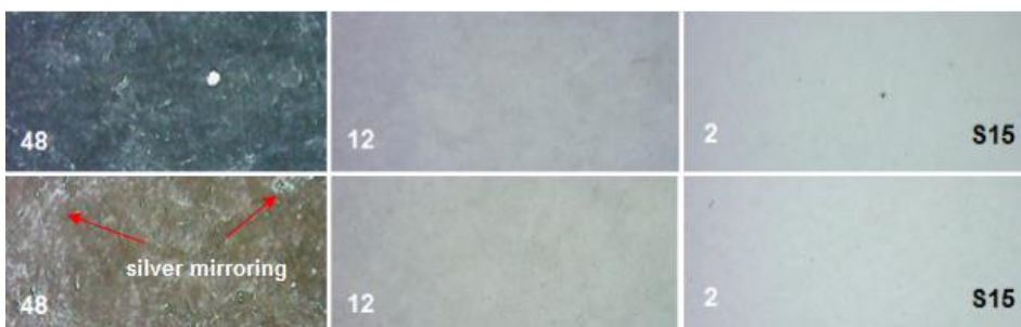
Fig. 3. Images taken by USB microscope showing the sample before exposure to hydrogen sulfide for 15 days (top) and after exposure (bottom). The red arrows point to mirrored areas.
