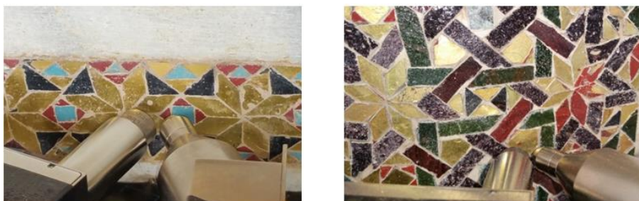
Fig. 10. XRF in situ analyses to identify the chromophores of mosaic glass tesserae.
