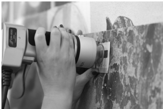
Fig. 2. Detail of the color measurement during the acquisition (detail of the head of the colorimeter) on one selected area using the acetate mask.
