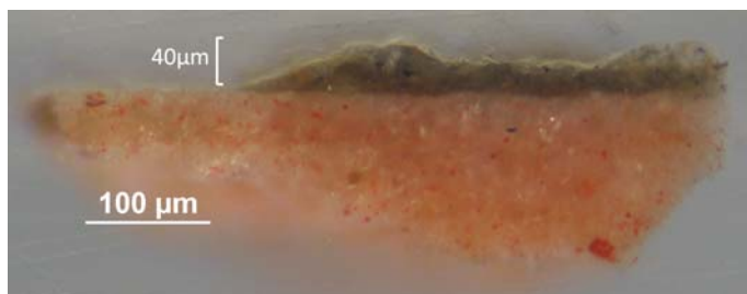
Fig. 3. Cross section of the sample taken from the boundary from a cleaned (SFR laser) and not cleaned surface
