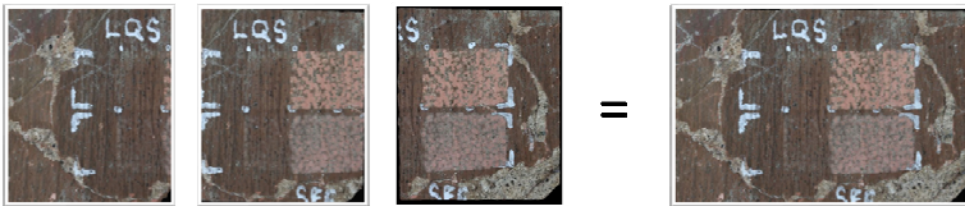
Fig. 7. Example of an arrangement of three 3D sub-models for LQS laser working area to obtain a single model
