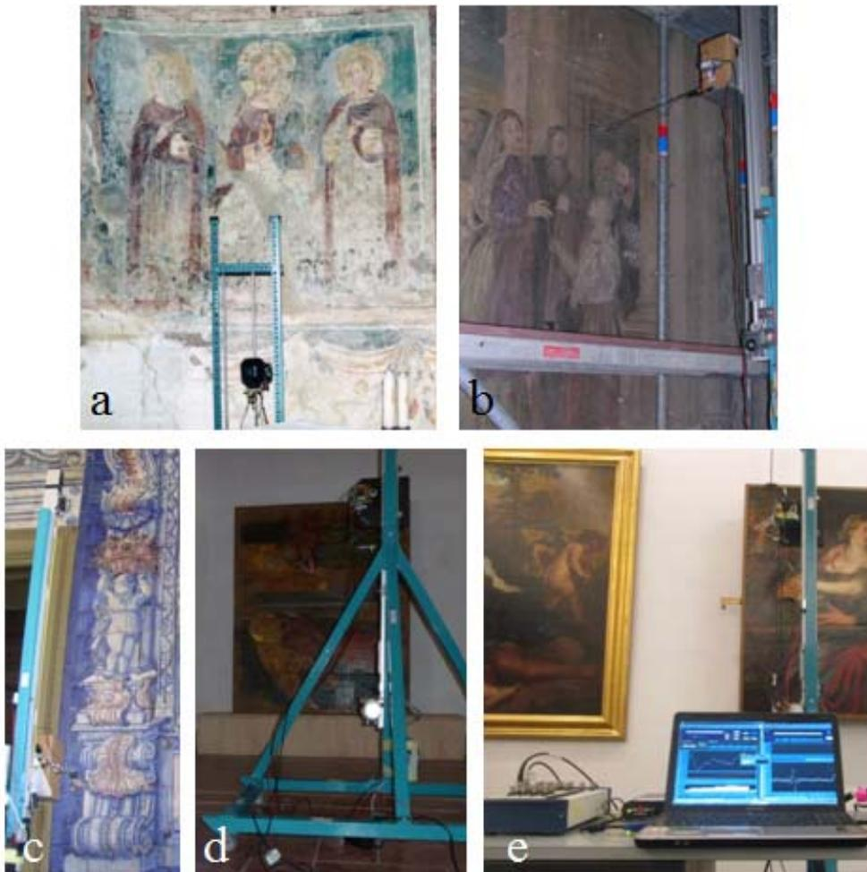
**Fig. 3.** Different configurations of the ACEADD system during on site experimentations: a – first in situ validation in the little Church of Santa Passera (Rome, 2001), b – the automated system during the analysis of the frescoes in Oratorio of San Rocco (Padua, 2011), c – in situ investigation of azulejo panels in the National Tile Museum (Lisbon, 2009), d and e – the device during the diagnostic tests of two panel paintings (Perugia and Genoa, 2011-2013).
