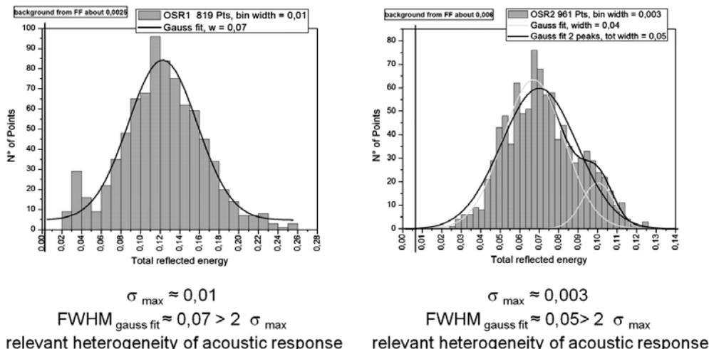
**Fig. 4.** Histogram of the acoustic response of the two maps OSR1 and OSR2, for the heterogeneity evaluation. The dispersion of the total reflection indicator, derived from the FWHM of the Gaussian fit, is compared with the uncertainty of measurement,  $\sigma_{\max}$ , obtained from the repeatability test.
